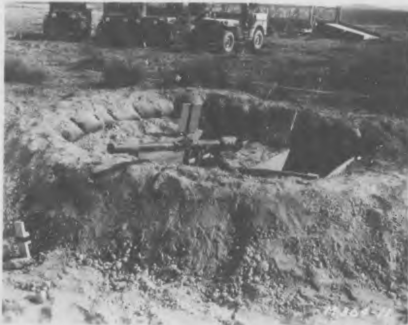
57 mm Recoilless Rifle - Before ↑ After Gun Blown 35 Yards Note: Burns ↓ on sand bags
